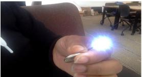
In order to solve the problem of making the LED light up using a 3v battery I put the long end of the LED leg (positive) with the plus sign of the LED. This created a working circuit.
